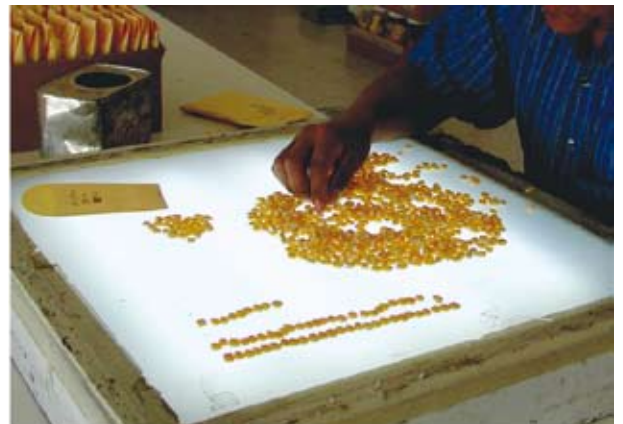
Figure 13. Screening maize kernels on a light table.
