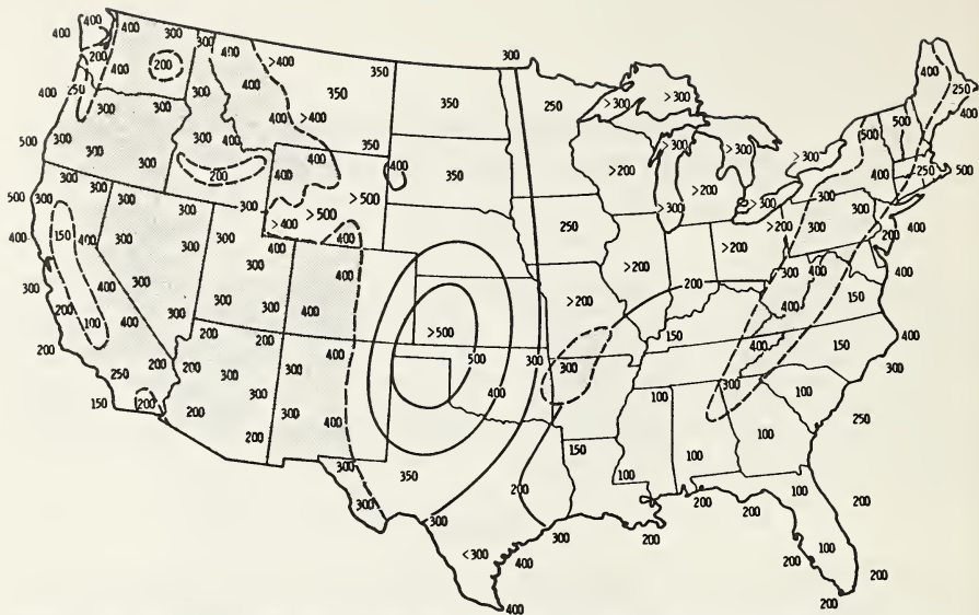
Figure 1.—Mean annual wind power (watts/m 2 ) estimated at 50 m above exposed areas. Over mountainous regions (shaded areas), the estimates are lower limits expected for exposed mountain tops and ridges (4).
