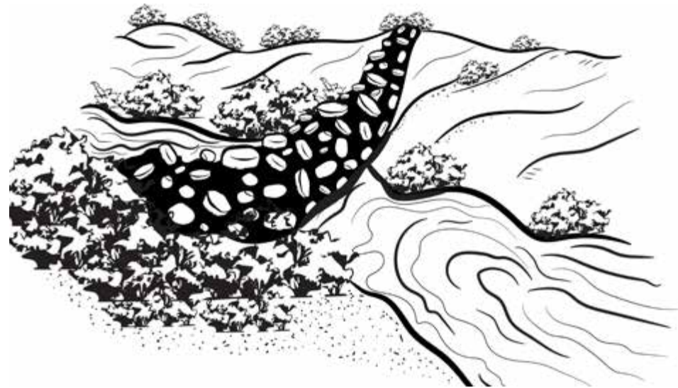
Construction of stone boulder embankment dam across a stream
