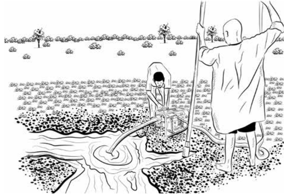
Connect pump for jetting with drilling pipe, lift water into the mud pit and ensure tight connections
