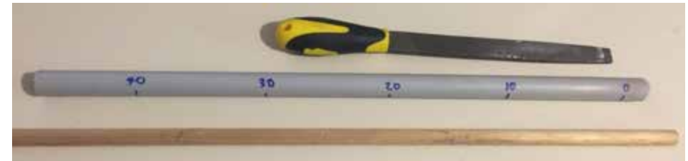
Figure 10.4. Sharpened 20mm pipe and 13mm dowel (Source: Richard Stirzaker)
