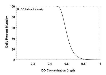
Figure 7. Dissolved Oxygen Growth Reduction (Panel A) and Induced Mortality (Panel B) Feedback Effects Used in the Bioenergetic Model.
