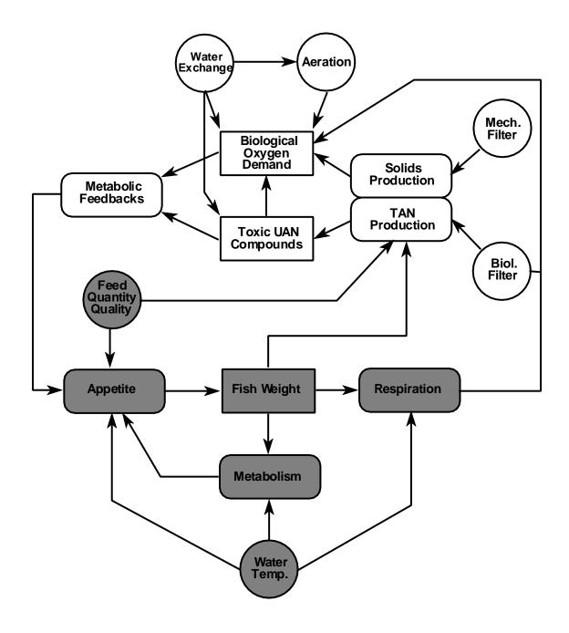
Figure 1. Conceptual Model of the Interactions Among Control Variables (circles), Process Variables (rounded polygons), and Storage Variables (rectangles) in a Recirculating Fish Production System (Shading denotes the bioenergetic components of the model).
