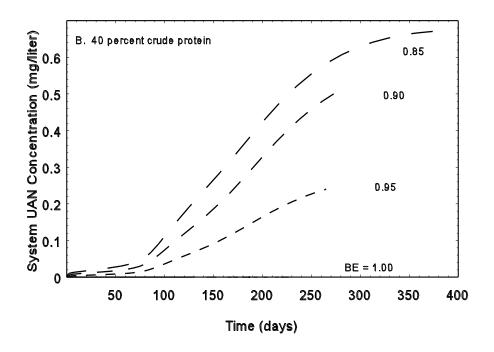
Figure 10. Effects of Different Feed Quality on Days-To-Harvest and System UAN Concentrations Given Varying Levels of Biological and Mechanical Filter Efficiency.
