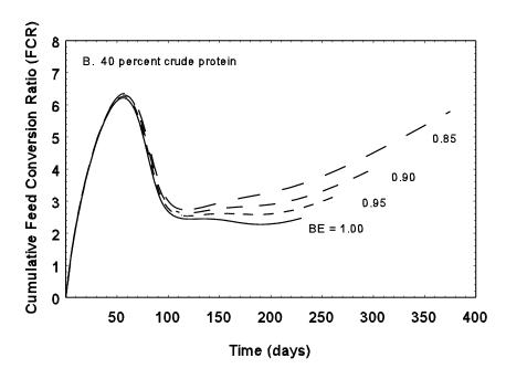
Figure 9. Effects of Different Feed Quality on Days-To-Harvest and Cumulative Feed Conversion Ratios (FCR) Given Varying Levels of Biological and Mechanical Filter Efficiency.
