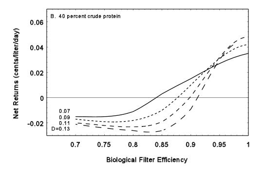
Figure 12. Simulated Daily Returns for Various Initial Stocking Levels (D) and Biological Filter Efficiencies Given a 20 Percent (Panel A) and 40 Percent (Panel B) Dietary Protein Feed.
