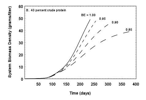
Figure 8. Effects of Different Feed Quality on Days-To-Harvest and Maximum System Biomass Density Given Varying Levels of Biological and Mechanical Filter Efficiency.
