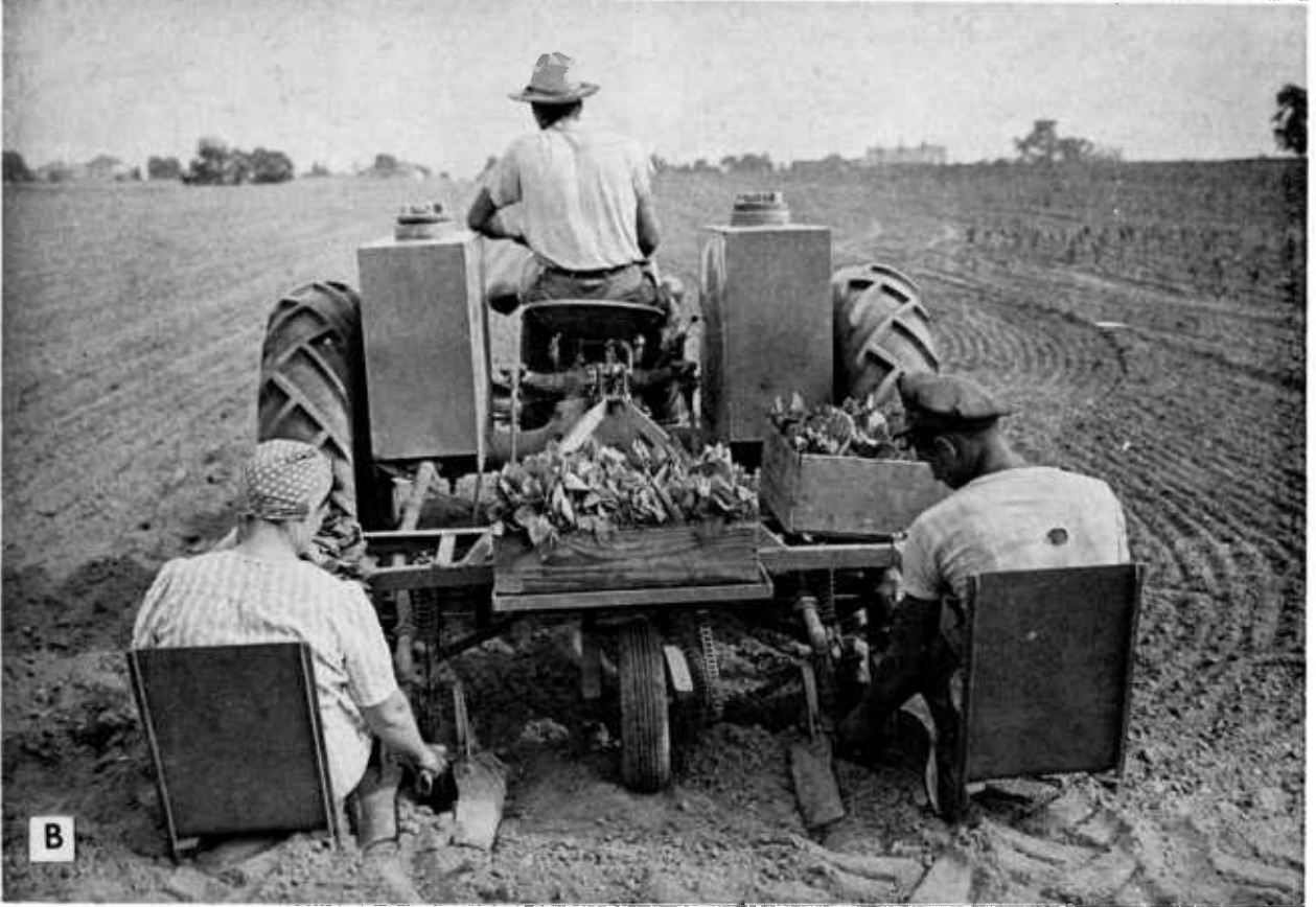
FIGURE 7.—Transplanting with tractor-drawn equipment: A , Single-row, power-lift transplanter used in setting burley tobacco in eastern Tennessee; B , two-row transplanter used in setting cigar filler plants in Pennsylvania.
