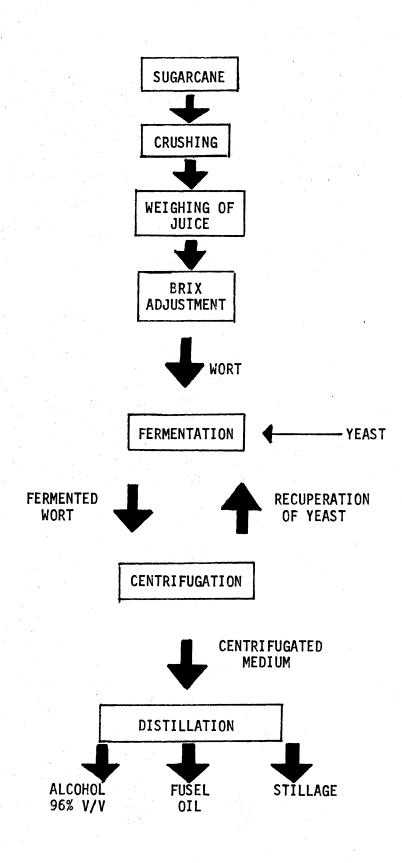
Figure 1. Flow Diagram -- Ethyl Alcohol Distillery
