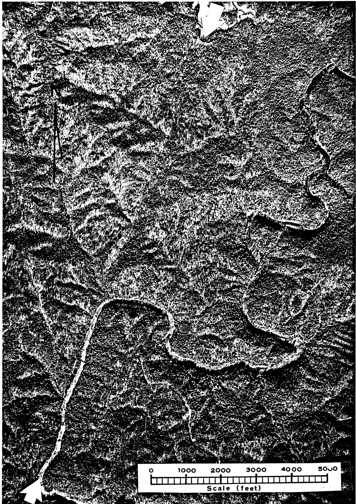
Figure 4. Coincident Alignment of Linear Drainage and Topographic Anomalies to Form a Prominent Lineament in Oconee County, South Carolina.
