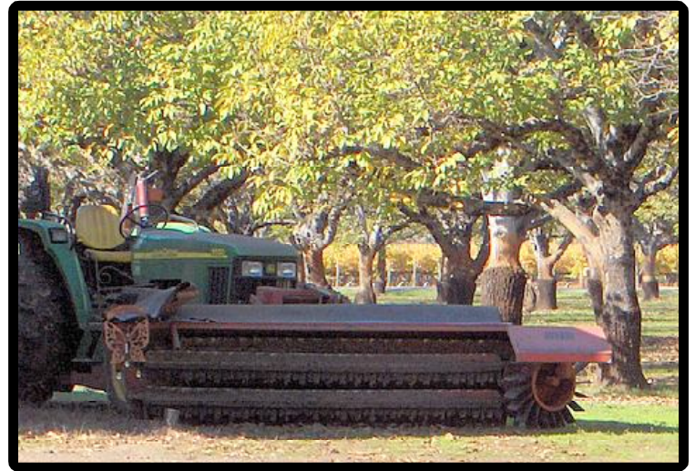
Mechanical picker: picks up the nuts and drops them into a bin
