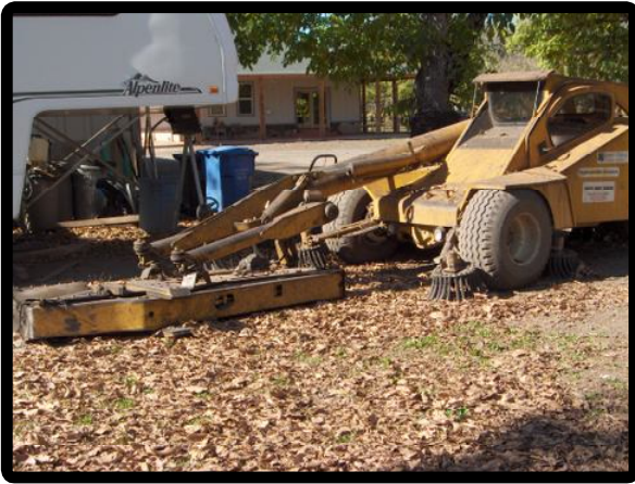
Tree shaker: grabs the tree trunk and shakes at a high frequency to knock the nuts to the ground.
