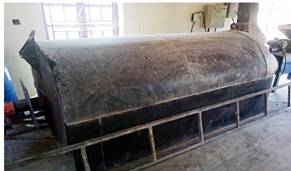
Plate 2: Flash drier that is run by electricity and diesel fuel
