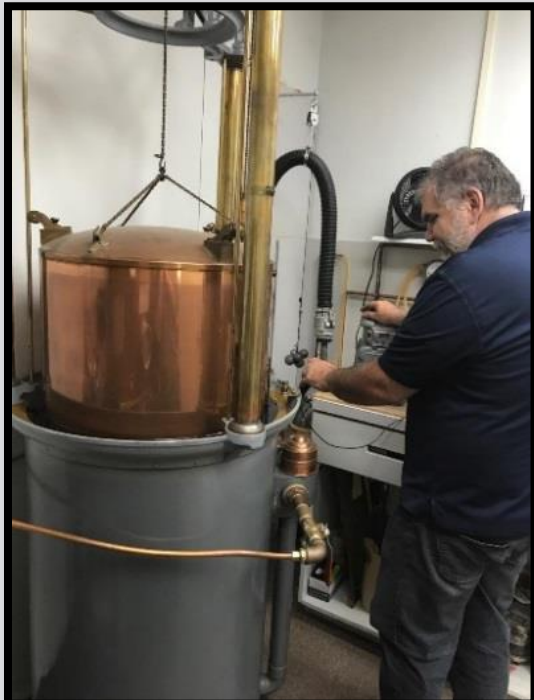
Left Photo: Dan Shrout testing gas utility submeters using a five cubic foot American Standard Bell Prover.
