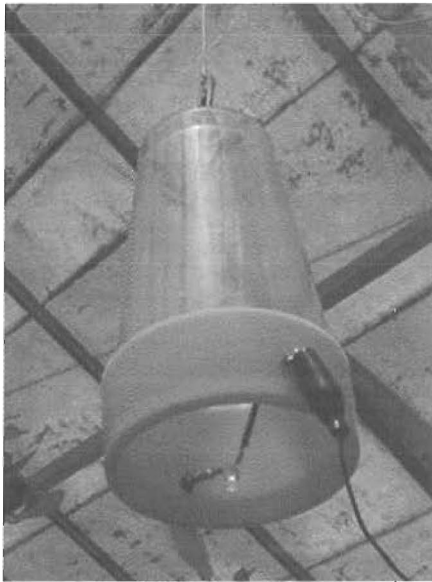
Figure 6. A CC trap equipped with a 530 nm lime green light-emitting diode for trapping insects in greenhouses.
