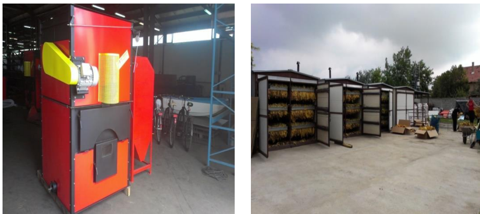
Picture 3. Heat generator and drier for tobacco
