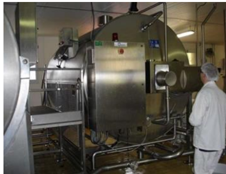
Figure 3. Horizontal device for cheese production
