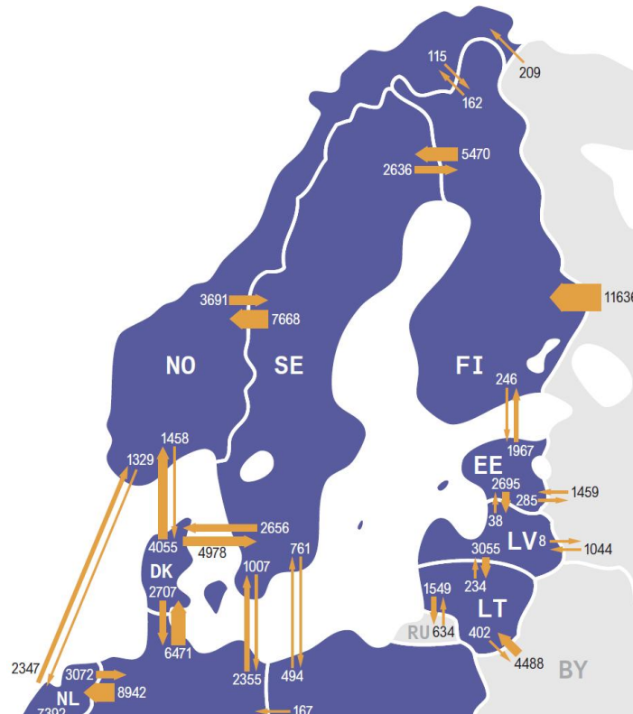
Fig. 1. The transmission of electricity between the countries in Northern Europe in 2010. (ENTSO 2011)
