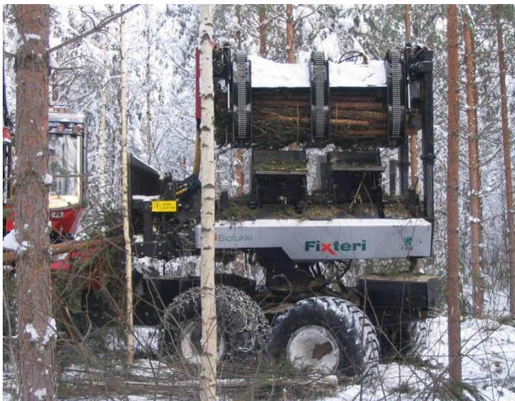
Figure 2. The accumulated bundle is lifted into the compressing chamber, in which it is compressed and wrapped using sisal string.
