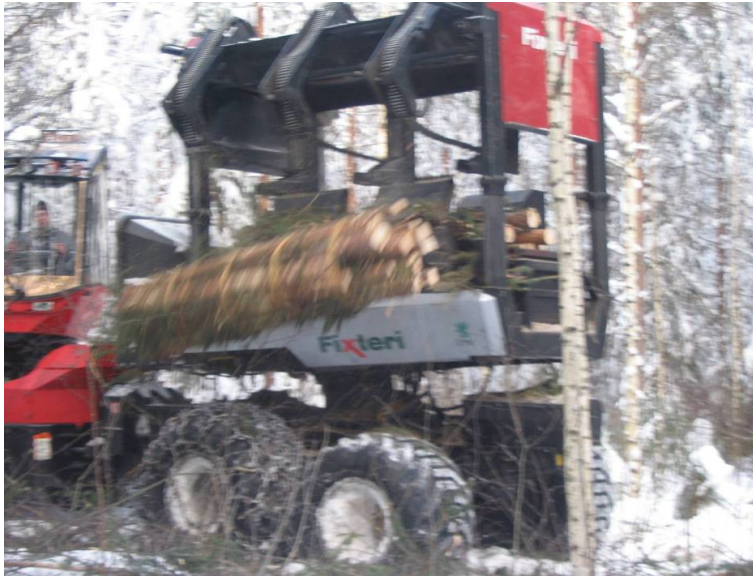
Figure 3. The compressed and wrapped bundle is dropped along the strip road.
