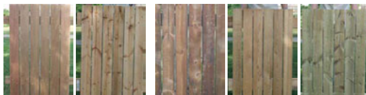
Figure 3. Five samples of decking used in the study (left to right: Untreated Ipé, Organic biocide treated Pine, Furfurylated Pine, Untreated Russian Larch, Copper treated Pine).
