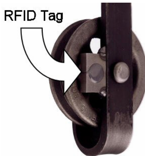
FIGURE 9. Gambrel radio frequency identification assembly
