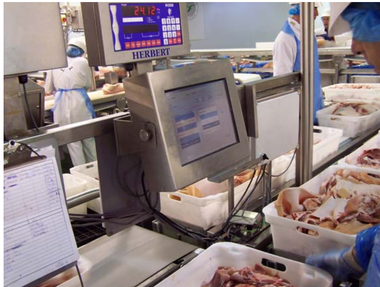
FIGURE 14. Computer monitors instructing meat cutters about how to process each ham
