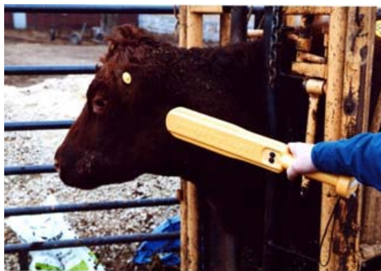
FIGURE 2. Hand scanner, Destron Technologies, Inc.
