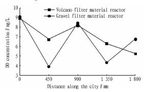
Fig. 4 DO concentration of filter bed in the first and third aeration filter bed
