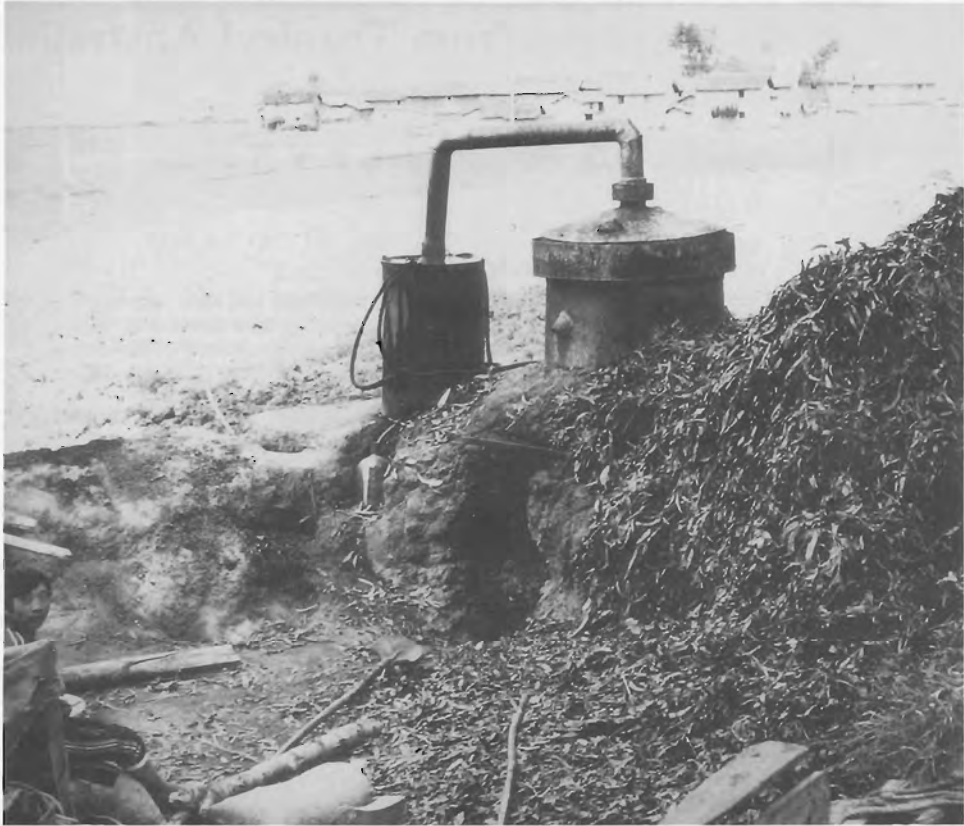
A small eucalypt oil distillation unit near Kunming, Yunnan province, People's Republic of China. The extraction of oils from Eucalyptus globulus leaves is a popular cottage industry in this region of China. Photographed April 1988.
