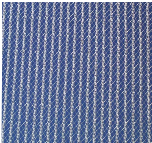
Figure 8. Close up of the 2 mm translucent monofilament fibre exclusion netting.
